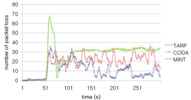
Fig. 9 Packet loss due to queue overflow
