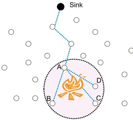
**Fig. 1** Event delivery in wireless sensor networks
