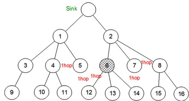
(a) Routing tree in sensor network.
